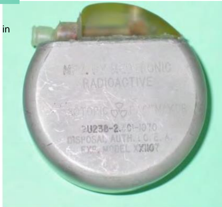
Figure 3 - This Medtronic nuclear pacemaker still “ticks” 35 years after it was manufactured.
