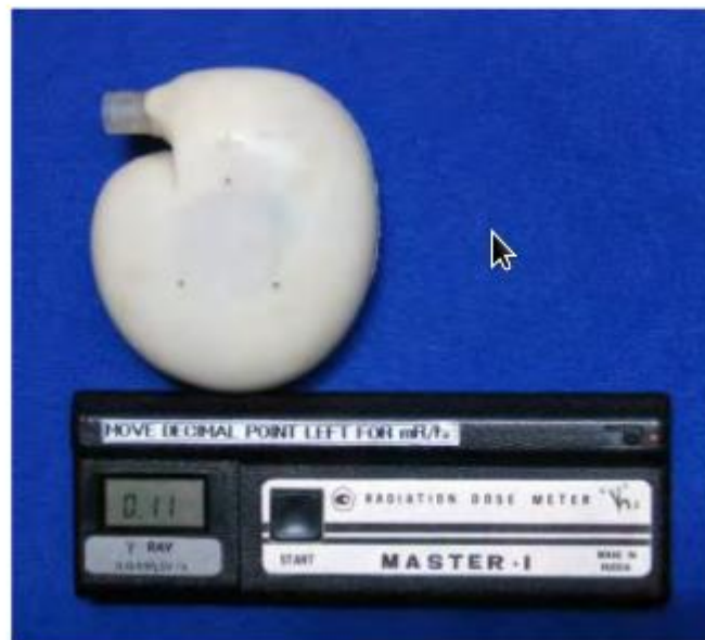
Figure 9 – No radiation above normal background could be detected from this CCC Betacel-powered nuclear pacemaker 30 years after it was manufactured.
