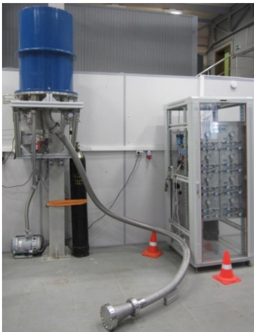
Fig. 3. General view of the thermosyphon system including LN 2 reservoir (on left), thermosyphon placed inside the bellow hose (in center) and the nitrogen fluid charging station (on right)
